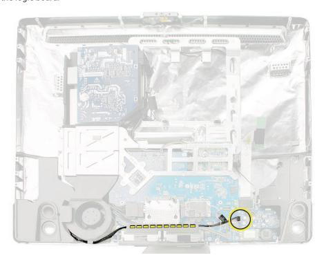
3. Lift the speaker out of the rear housing.
